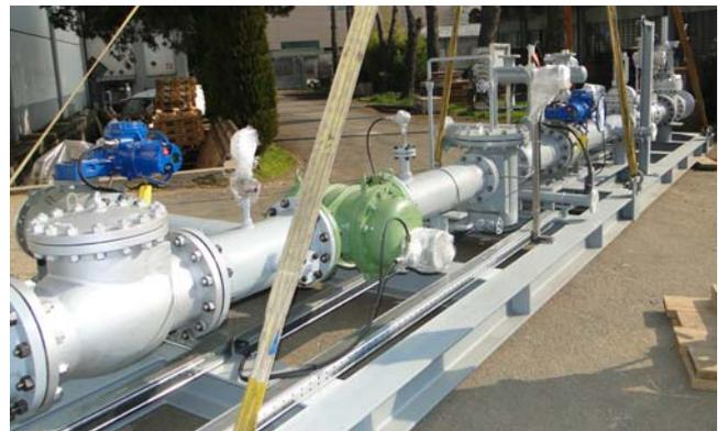
Reduction, filtering and measure fuel skid
